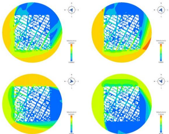
Figure 11: Velocity contours for wind conditions 13–16.
