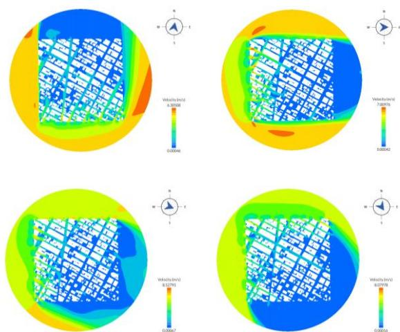
Figure 10: Velocity contours for wind conditions 9–12.
