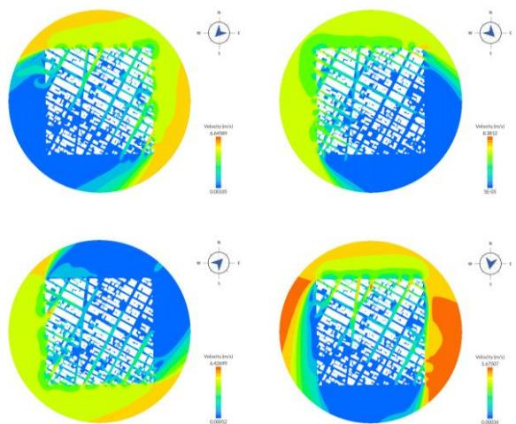
*Figure 8: Velocity contours for wind conditions 1–4.*
