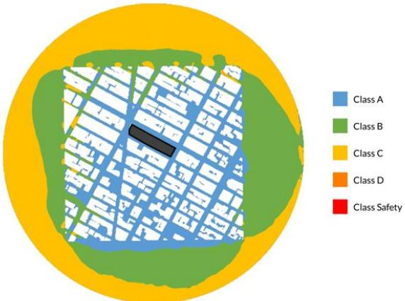
Figure 12: Comfort plot at 1.6m above ground.
