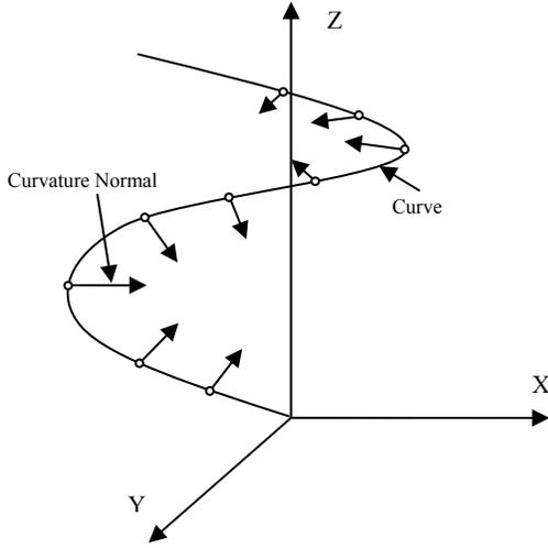
Figure 2. Curvature normal of curve
