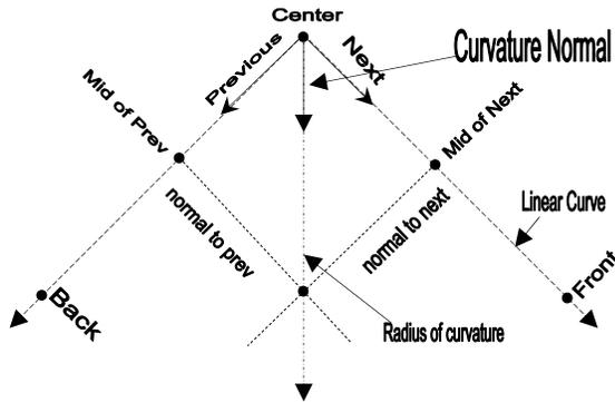
Figure 3. Curvature normal computation
