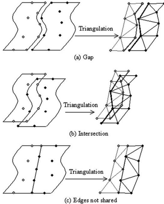
Figure 1, Error in CAD data for grid generation difficult.
