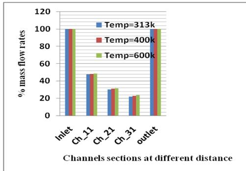
“Fig.11” % Mass flow rates variation at Re=122 and temp=313k, 400k, 600k
