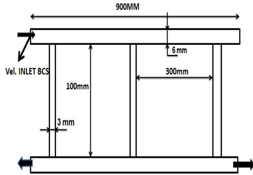
“Fig.1.” U and Z- turn configurations
