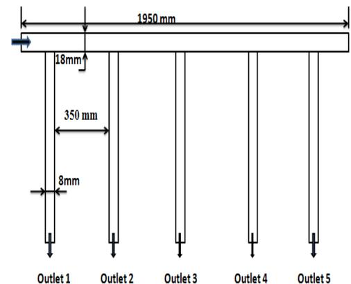
“Fig. 4.” Experimental set up for validation.
