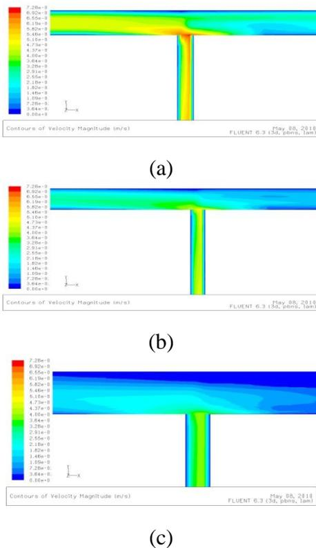
“Fig. 6.” Velocity contours (Re=1759) at section (a) 11, (b) 12 and (c) 13
