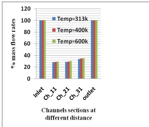
“Fig.12” % Mass flow rates variation at Re=122 and temp=313k, 400k, 600k
