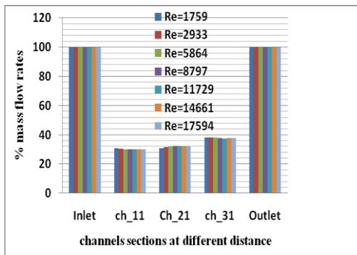
“Fig.9.” Effect of Re on percentage mass flow rate for Z-turn configuration
