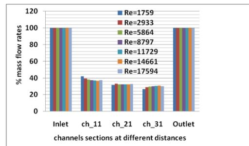
“Fig.8.” Effect of Re on percentage mass flow rate for U-turn configuration
