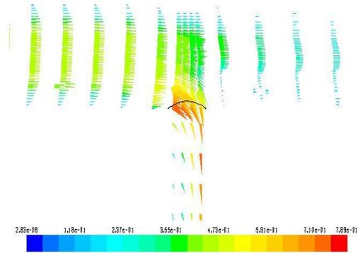
“Fig. 7.” Velocity vectors (Re=1759) at section (a) 11
