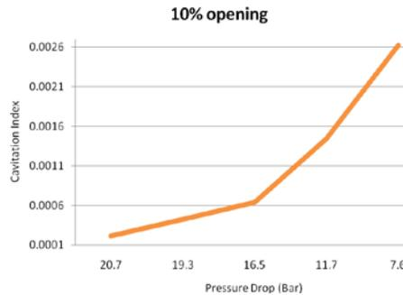
Fig. 8 Cavitation index for 10 percent opening and varying pressure drop
