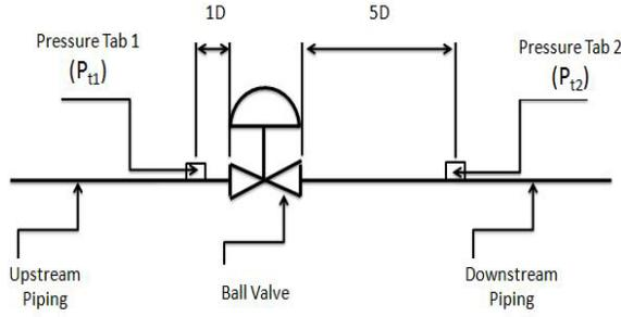
Fig. 2 Schematic diagram of ball valve and piping system
