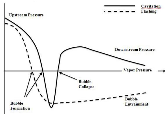
Fig. 3 Pressure variation for cavitation and flashing process
