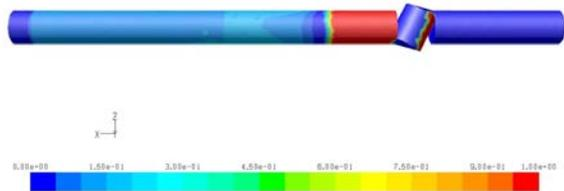
Fig. 7 Volume fraction of vapor phase for 30 percent opening
