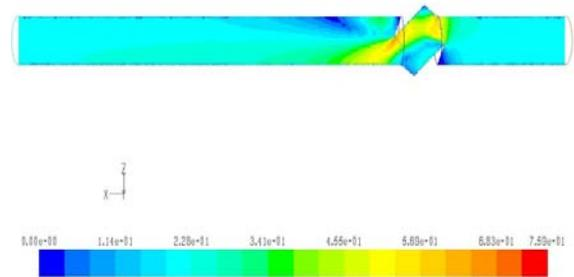
Fig. 4 Velocity contour plot for 60 percent opening
