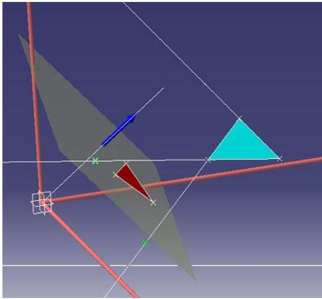
After performing the intersection, points on surfaces are displayed which form actual boundaries, for face, which separates the surfaces from each other. The faces of the target and the tool bodies are intersected with each other to produce new edges where they meet. These edges divide the faces of each body into facesets which are either inside, outside, or on the boundary of, the other bodies.
