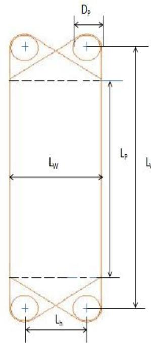
“Fig.3” Simplified channel plates geometry
