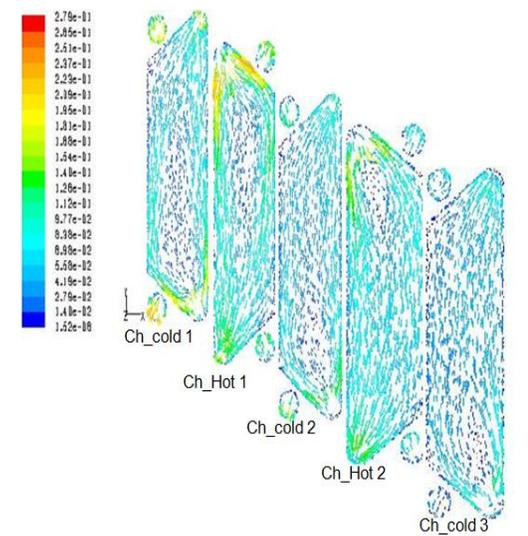
“Fig.16” (c) Velocity contours and vectors at  $Re=10000$
