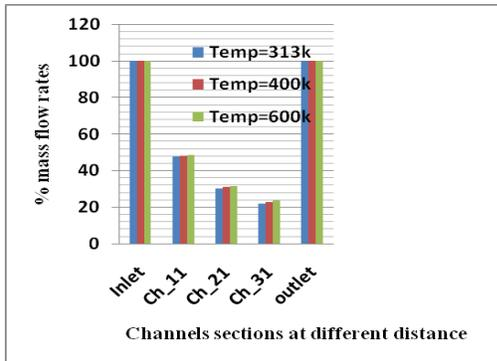
“Fig.13” % Mass flow rates at Re=122 and temp=313k, 400k, 600k (U- turn flow configuration)
