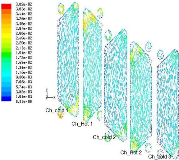
“Fig.16” (a) Velocity contours and vectors at  $Re=1500$
