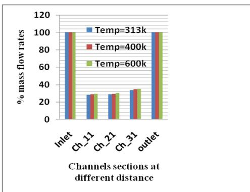
“Fig.14” % Mass flow rates at Re=122 and temp=313k, 400k, 600k (Z- turn flow configuration)
