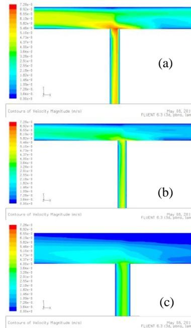
“Fig.8” Velocity contours (Re=1759) at section (a) 11, (b) 12 and (c) 13
