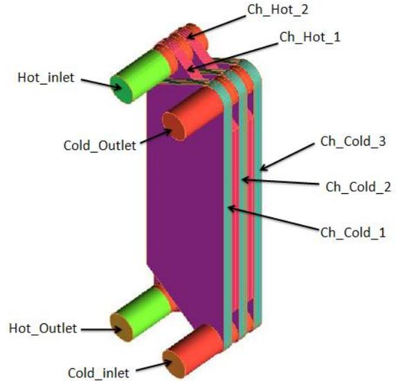
“Fig.15” Designation of channel sections for simplified model of PHE
