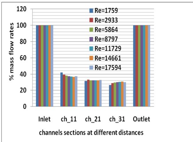
“Fig.10” Effect of Re on % mass flow rate for U-turn configuration
