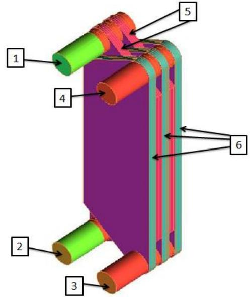
“Fig.2” Simplified solid model of PHE, (1) Hot inlet port, (2) Hot outlet port, (3) Cold inlet port, (4) Cold outlet port, (5) Hot channels and (6) Cold channels
