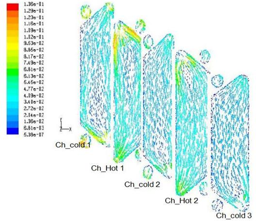
“Fig.16” (b) Velocity contours and vectors at  $Re=5000$
