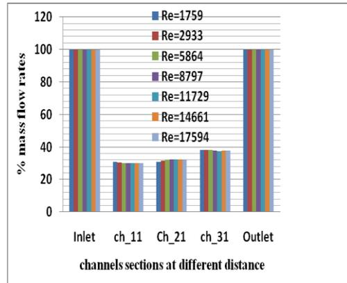
“Fig.11” Effect of Re on % mass flow rate for Z-turn configuration
